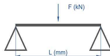
Point load applied to an area of 50x50 mm
